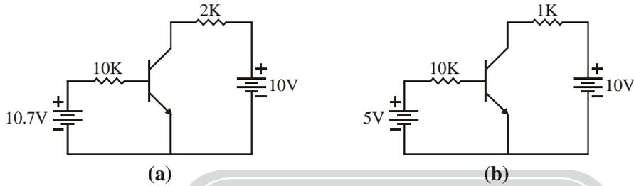
If the transistors in Figures (a) and (b) have current gain ( $\beta_{dc}$ ) of 100 and 10 respectively, then they operate in the
